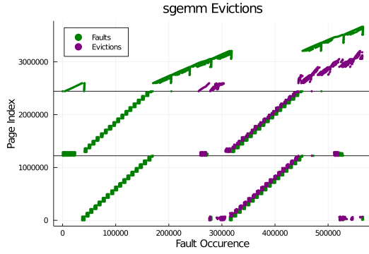
Fig. 8: This figure demonstrates sgemm with a problem size that requires approximately 120% of GPU memory. Notably, we show evictions at the relative time step they are issued. Evict and re-fault is a worst-case performance scenario.
